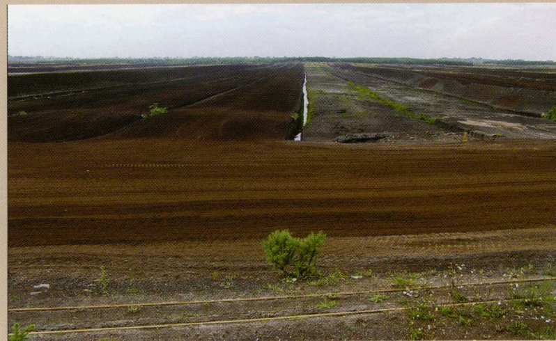
Cutaway peatlands in production showing drains every 15 m and, below, 'peat exhausted' bays beside peat field still in production (Noggus).
